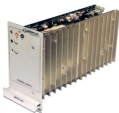
BAP 236-EH plug-in module (200W) 3U x 14HP x 220mm
